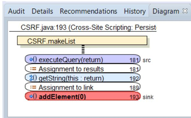
For dataflow issues, the trace starts with the first function to call the taint source, then traces the calls to the source (blue node), and ends the trace at the sink (red node). In the diagram, the source (src) and sink nodes are also labeled. A red X on a vertical axis indicates that the called function finished executing.
