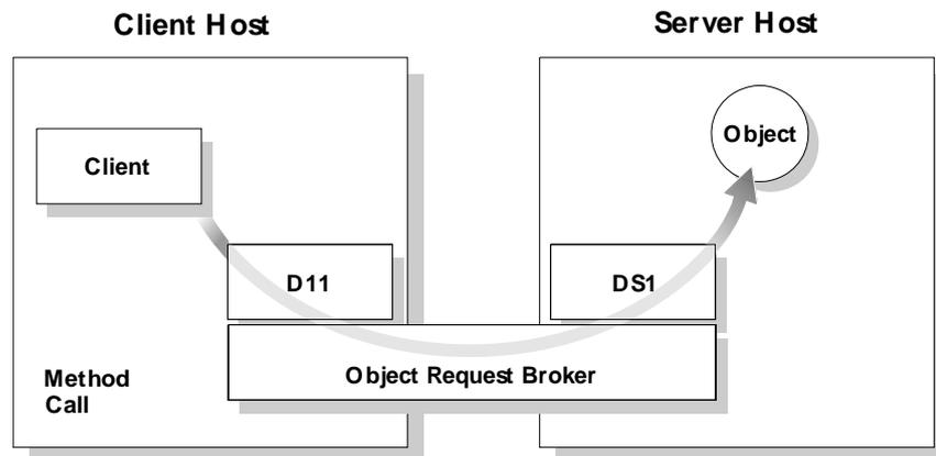
**Figure 4:** Method Call Using the DII and DSI
