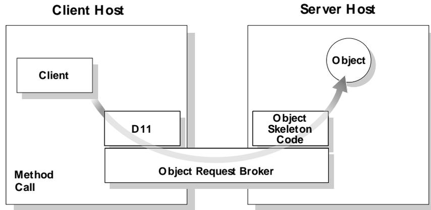
**Figure 3:** Client Invoking a Method Using the DII
